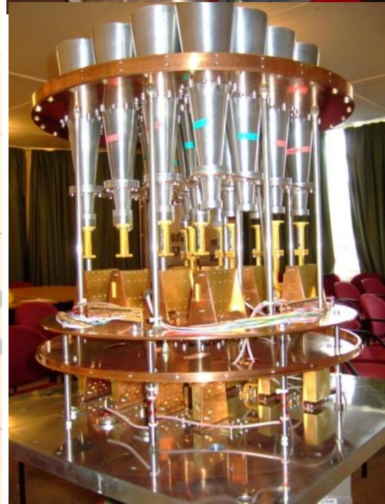
Multi beam receiver OCRA-f on RT32m, at 30 GHz
